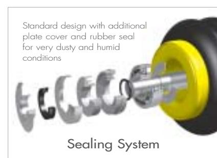
To meet customer requirements Transroll offers three different designs of shaft-sealing system.
